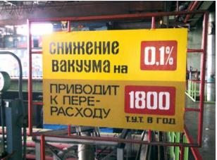
Placard in heat power station turbine workshop. The text is: 0,1% vacuum loss cause excess 1800 tons of standard coal fuel
